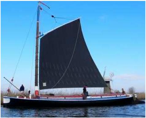
This has been a massive project that has taken Albion from the point where she was in appalling condition and leaking badly to one where she is in excellent condition structurally, with stiffer. better shape. To round things off her ballast has been increased a little to set her lower in the water (her natural position
