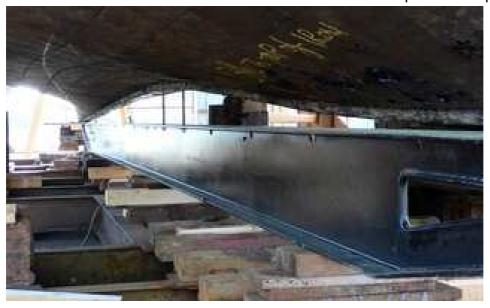
the slip. The procedure was brutally simple. Her old wooden keel was sawn off, bolts old drawn and a template of the boltholes new was fastened to the underside of her hog. All boltholes new were drilled and new keel/girder was
