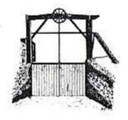
Guillotine staunches usually consisted of a shutter or clough raised vertically out of the water by chains. That at Bone Mill, on the Nar, (left) was raised by the operator climbing the ladder and turning an iron wheel to open the gate. On
