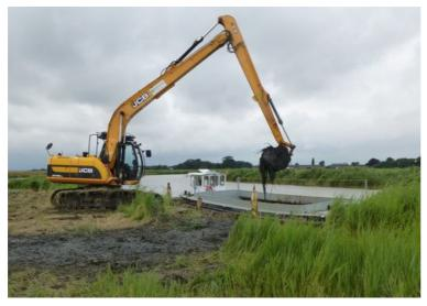
Another development is the retirement of the old steelhulled barge with a crane mounted on it; this has been replaced by a versatile long reach excavator which will sit on linkflotes and dredge using a new hydraulic clam shell Over the last four bucket. years the Authority has purchased three of the long hydraulic excavators and a set of four linkflotes.
